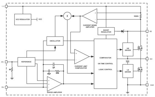
30V,3A synchronous Step-Down Converter
